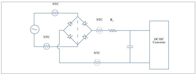
Figure3 : Surge Current Limiting Circuit For Switch Mode Power Supply.
