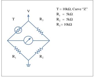
Figure 2: Wheatstone Bridge - Voltage Mode
