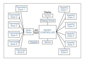
Figure 1: Microcontroller System
