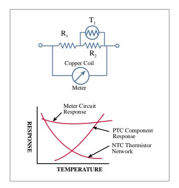
Figure 24: Temperature Compensation
